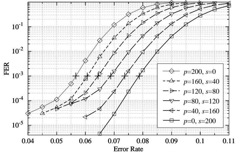
Fig. 3. FER over the BSC for a binary LDPC code of length  $2 \times 10^3$  bits and rate  $R_0 = 1/2$ . Several curves have been simulated for different proportions of punctured and shortened symbols, with  $d = 200$ . The distribution of punctured symbols has been chosen according to a pattern previously estimated as proposed in Ref. [23].
