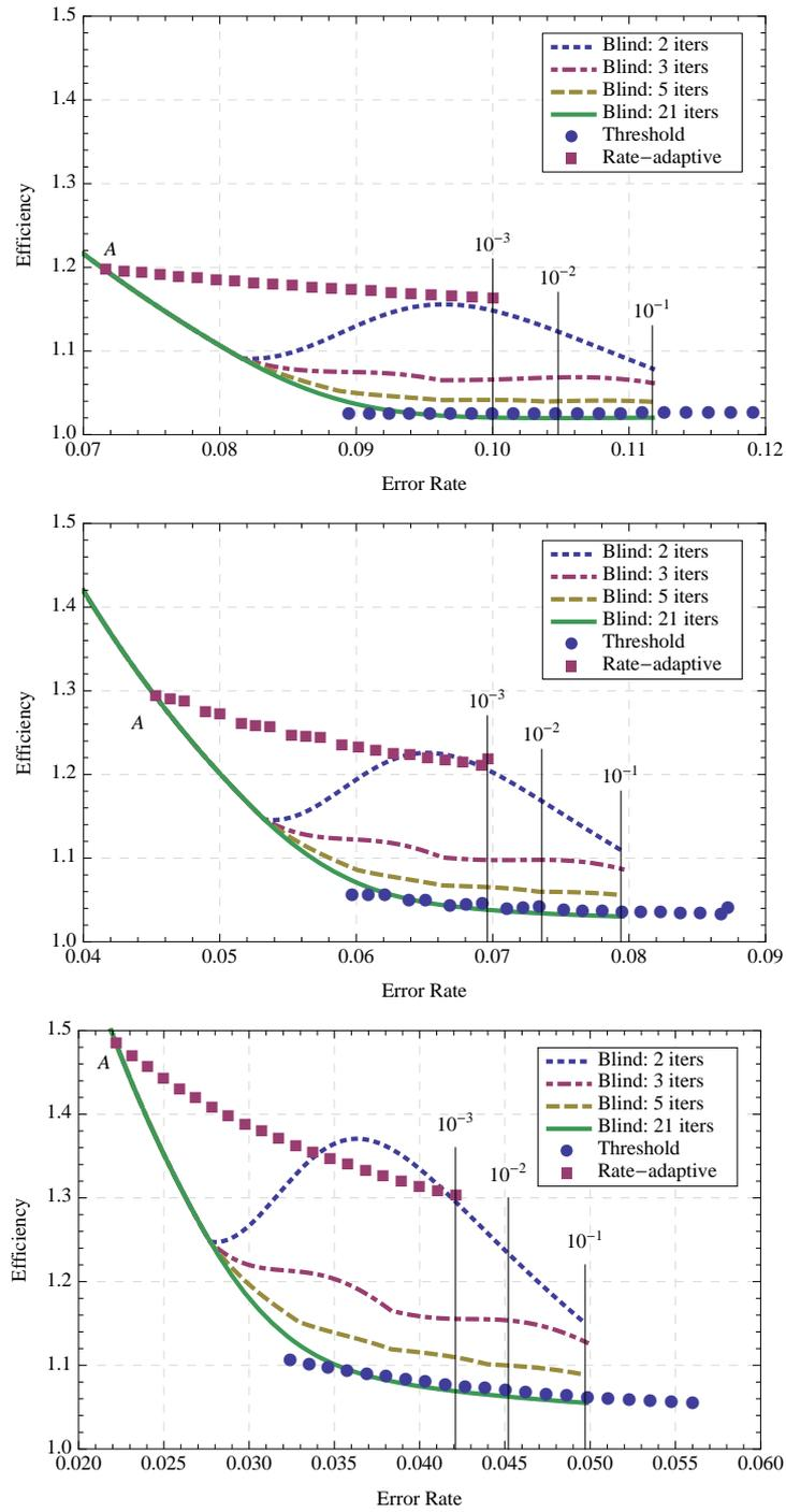
Fig. 5. The estimated efficiency (Gaussian approximation) of the rate adaptive protocol is compared to the efficiency of the blind protocol for short codes ( $2 \times 10^3$  bits length). Three coding rates are used to cover the error range [2.5%, 11%]. A detailed description is given in the text.
