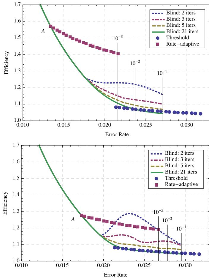
Fig. 6. Estimated efficiency curves, as in Fig. 5, for a coding rate  $R = 0,8$  and different codeword length,  $2 \times 10^3$  (top) and  $10^4$  (down) bits length. A detailed description is given in text.
