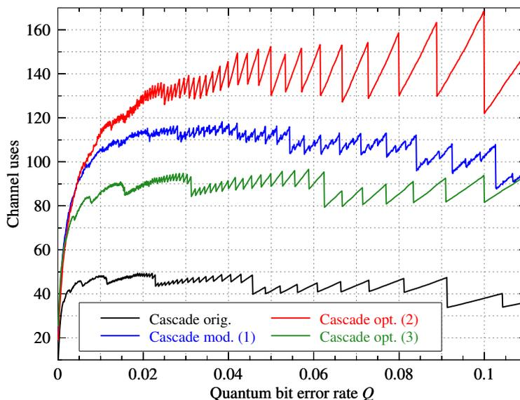
Fig. 9. Channel uses of the original *Cascade* (black) and three modified versions: (1) the modified protocol proposed in [10] (blue), (2) the version using the optimized parameters suggested in [19] (red), and (3) the version proposed here using 16 passes (green). More details are given in the text.
