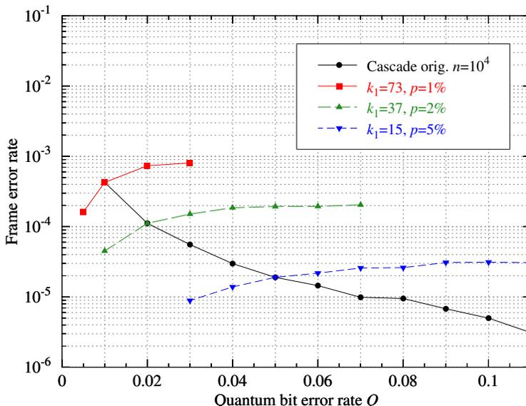
Fig. 7. Frame error rate (failure probability) as a function of the quantum bit error rate when  $k_1$  is fixed over a larger interval of  $Q$  than originally proposed [6]. For comparison, also the frame error rate of this original **Cascade** protocol is shown.
