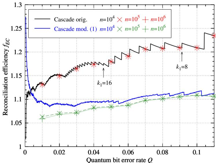
Fig. 1. Comparison of the average reconciliation efficiency as a function of the quantum bit error rate  $Q$  for the original **Cascade** protocol [6] and the version of [10] (i.e., modified version (1) throughout this paper). The length of the frames used is denoted by  $n$ .
