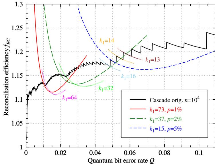
Fig. 6. Average reconciliation efficiency,  $f_{EC}$ , as function of the quantum bit error rate when  $k_1$  is fixed over a larger interval of  $Q$  than originally proposed [6]. For comparison also the efficiency of the original Cascade protocol [6] is shown.
