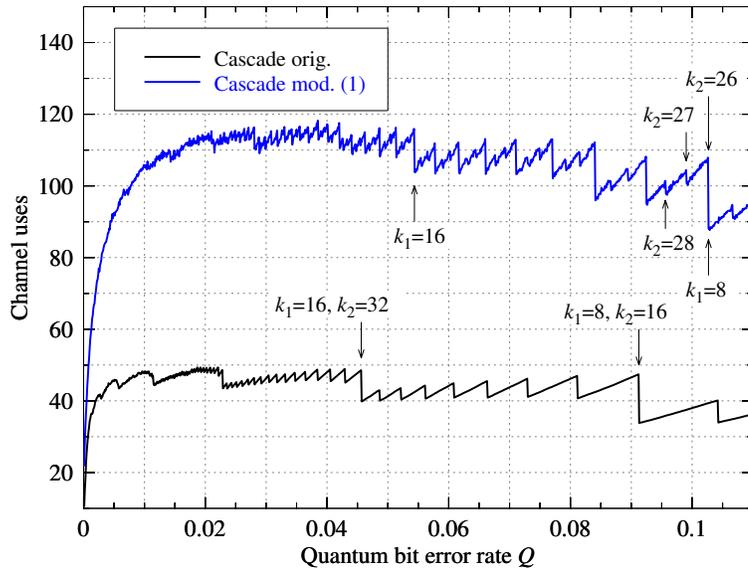
Fig. 2. Comparison of the number of channel uses as a function of the quantum bit error rate  $Q$  for the original **Cascade** protocol [6] and the version (mod. (1)) of [10].
