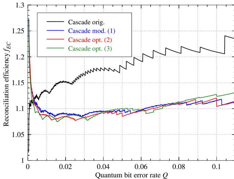
Fig. 8. Average reconciliation efficiency,  $f_{EC}$ , of the original **Cascade** (black) and three modified versions: (1) the modified protocol proposed in [10] (blue), (2) the version using the optimized parameters suggested in [19] (red), and (3) the version proposed here using 16 passes (green). More details are given in the text.
