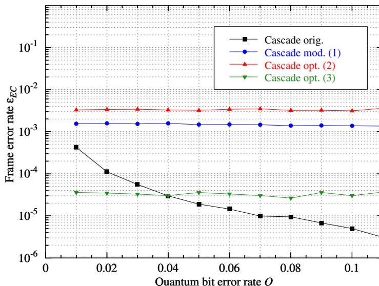
Fig. 10. Frame error rate (failure probability) of the original **Cascade** (black) and three modified versions: (1) the modified protocol proposed in [10] (blue), (2) the version using the optimized parameters suggested in [19] (red), and (3) the version proposed here using 16 passes (green). More details are given in the text.
