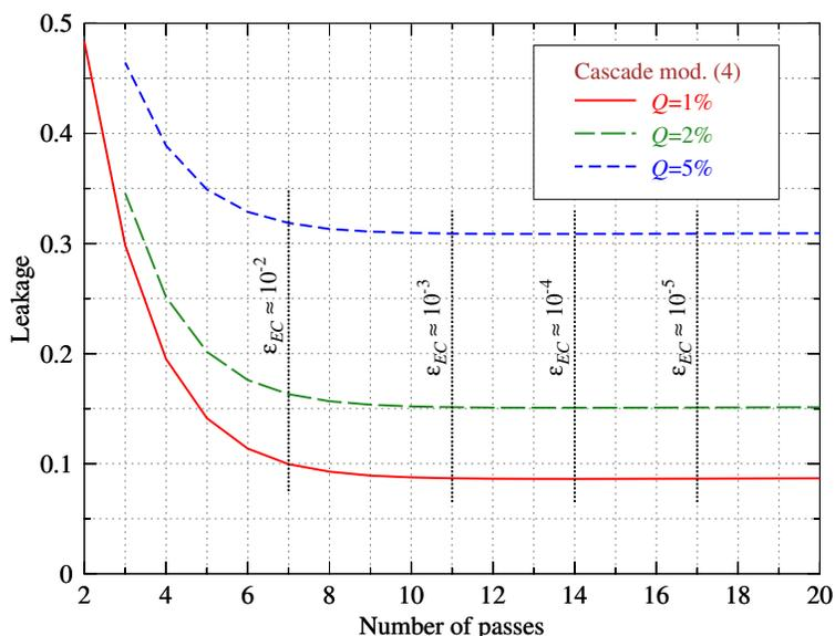
Fig. 12. Information leakage as a function of the number of passes in the proposed modification of **Cascade** utilizing subblock reuse, labeled with (4) in Fig. 11.
