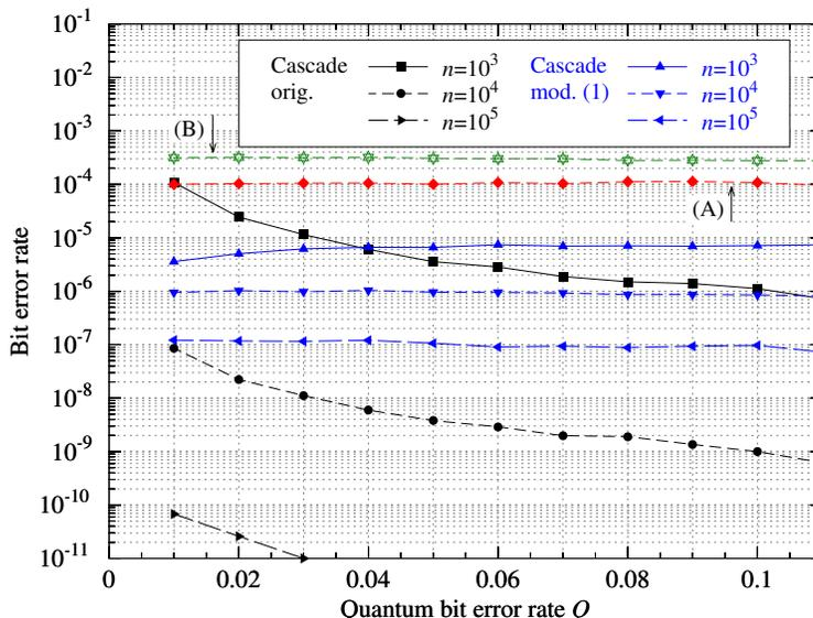
Fig. 5. Bit error rate (residual error) as a function of the quantum bit error rate for the original Cascade protocol [6] and the version (mod. (1)) of [10]. The curves labeled (A) and (B) correspond to the bit error rate after the first two passes of the original Cascade (A) and two passes in the modified one without BICONF (B).
